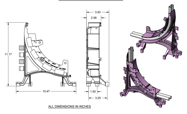
The PEXRITE® #708 POP-UP™ supports up to three 3/8" O.D. or two 1-1/8" O.D. flexible tubing lines (PEX or softer copper). Ideal for positioning tubing prior to concrete slab pouring. For elevated slabs, nail bracket to form decking or edge form. For slab-on-grade (ground work), secure bracket with #4 rebar driven into the ground.
