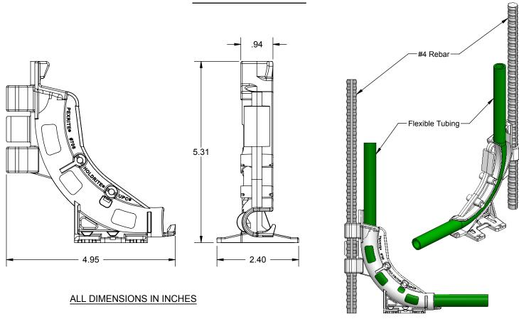
The PEXRITE® #706 supports one 3/8" - 5/8" O.D. flexible tubing line (PEX or soft copper). Ideal for positioning tubing at 90 $^\circ$  prior to concrete slab pouring. For slab-on-grade (ground work), secure bracket with #4 rebar driven into the ground.
