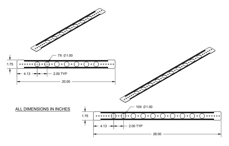
The LOCKRITE™ #601-20 and #601-26 are 20 gage galvanized steel brackets designed exclusively to support CPVC piping. Rolled edges provide added strength. Works exclusively with our glueable HOLDRITE® #604 (1/2") or #605 (3/4") inserts. Inserts snaps into brackets.
