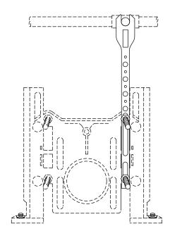
The HOLDRITE® #114-CR is a Copper-Bonded™ steel bracket with two slots for securely mounting upright to the carrier unit. The top end has a single 1-1/8" extruded slot for soldering 1" copper flush valve supply line. Secures the flush valve 4-1/2" from the carrier center and 14" above the top carrier mounting bolt. Excellent for pre-fab. Supports flush valve rough-in prior to wall framing. When soldering, heat the pipe, not the bracket.
