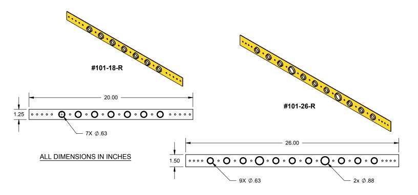
The HOLDRITE #101-18-R and #101-26-R are Copper-Bonded™ steel brackets with extruded holes. The #101-18-R has 5/8" holes on 2" centers. The #101-26-R has 5/8" holes on 2" centers and 2 - 7/8" holes on 8" centers. Each to support 1/2" or 3/4" copper tubing. The #101-18-R and #101-26-R position copper water supplies for sinks, water closets, and other fixtures. When soldering, heat the pipe, not the bracket.
