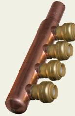
Manifolds are traditionally used in PEX systems, but this new SharkBite manifold will allow easy incorporation into copper or CPVC systems. Use SharkBite push fittings to install these manifolds anywhere in a plumbing system. All manifolds have a 1" trunk with 3/4" tube inlets & outlets and 1/2" push-fit ports (2" on center).
