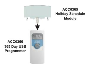
**(B)** Once connected, the USB Programmer LED will flash **green** 5 times. A **red** flash indicates an error has occurred. Try reconnecting the module.
