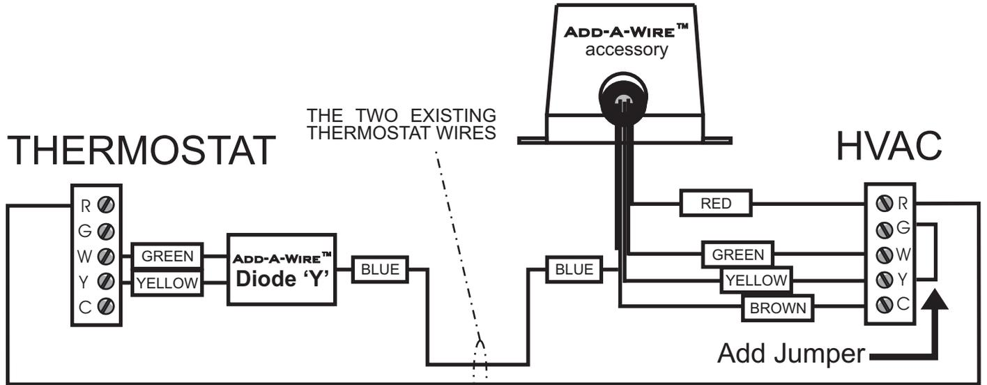
2 existing wires with **ADD-A-WIRE™** to accommodate heating and cooling. No independent fan switching. A jumper is required across G & Y.
