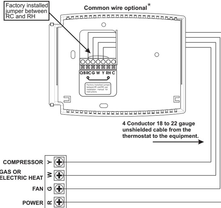
\* Common wire is optional in all installations. If a common wire is not used the thermostat must be powered by two AA alkaline batteries. These batteries must be replaced (page 6) each year or when the Low Battery indicator is displayed (page 3).
