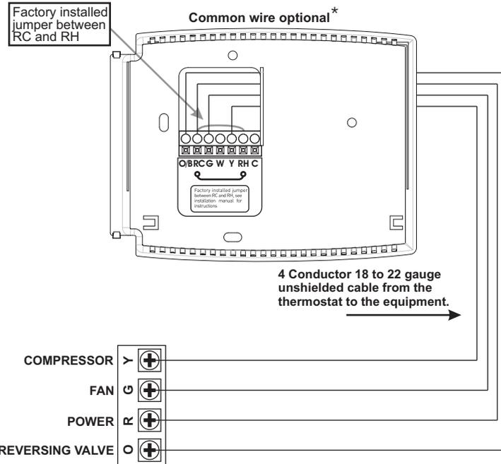
\* Common wire is optional in all installations. If a common wire is not used the thermostat must be powered by two AA alkaline batteries. These batteries must be replaced (page 6) each year or when the Low Battery indicator is displayed (page 3).
