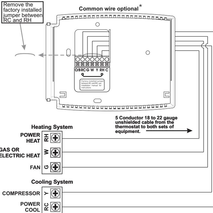
\* If a common wire is used it must be connected to the furnace common terminal. If a common wire is not used the thermostat must be powered by two AA alkaline batteries. These batteries must be replaced (page 6) each year or when the Low Battery indicator is displayed (page 3).
