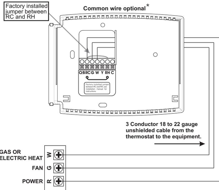
\* Common wire is optional in all installations. If a common wire is not used the thermostat must be powered by two AA alkaline batteries. These batteries must be replaced (page 6) each year or when the Low Battery indicator is displayed (page 3).
