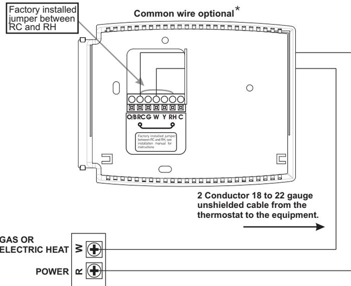
\* Common wire is optional in all installations. If a common wire is not used the thermostat must be powered by two AA alkaline batteries. These batteries must be replaced (page 6) each year or when the Low Battery indicator is displayed (page 3).
