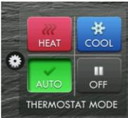
**AUTO-CHANGEOVER MODE** - Pressing the WARMER or COOLER buttons in Auto mode will adjust **both** the heat and cool setpoints simultaneously. To adjust heat and cool setpoints individually, choose HEAT mode to adjust the heat setpoint and COOL mode to adjust the cool setpoint, then return to AUTO mode.
