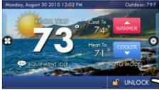
When the thermostat is locked, the bottom bar of the display will show:
