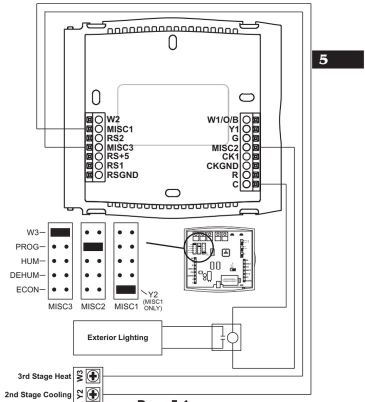
Adding a Humidification System\* (MISC1), Dehumidification System\* (MISC2), and controlling an Economizer (MISC3).
