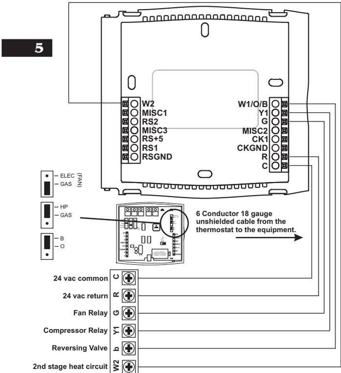
**Adding a 2nd Stage of Cooling (MISC1), Exterior Lighting System (MISC2), and 3rd Stage of Heating (MISC3)**
