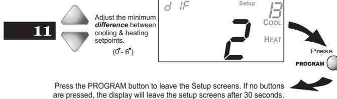
**Note:** To increase the spread between the heating and cooling setpoints, press the MODE button until only the heat setpoint is displayed. Adjust the desired setpoint. Press the MODE button until only the cool setpoint is displayed. Adjust the desired setpoint. Press the MODE button again to enter the Auto-Changeover mode where both the heat and cool setpoints are displayed.
