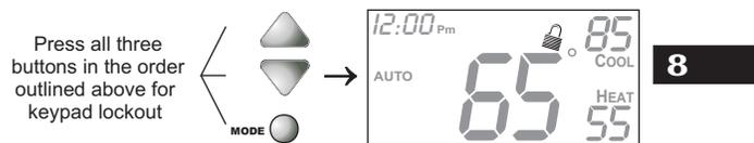
To **unlock** the keypad, press and hold the MODE button. While holding the MODE button, press the UP and DOWN buttons together. The
