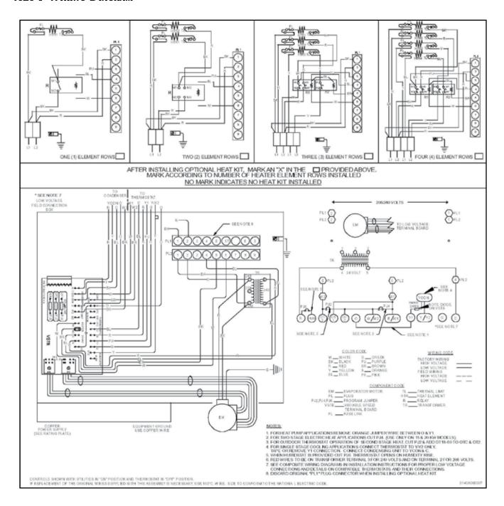
Wiring is subject to change. Always refer to the wiring diagram or the unit for the most up-to-date wiring.
