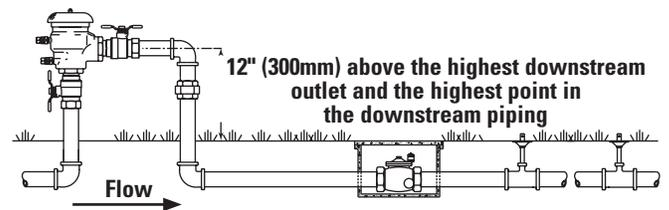
Thermal water expansion and/or water hammer down stream of the backflow preventer can cause pressure increases. Excessive pressure should be eliminated to avoid possible damage to the system and assembly.
