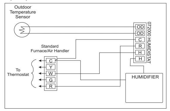
The diagram below shows the wiring for the ULTRA-ZONE Model S-2000 and S-2020 Steam Humidifiers
