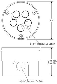
The PM-HSC5 is a slab mounted snow detector, designed to be embedded in a concrete slab, or other masonry material.
