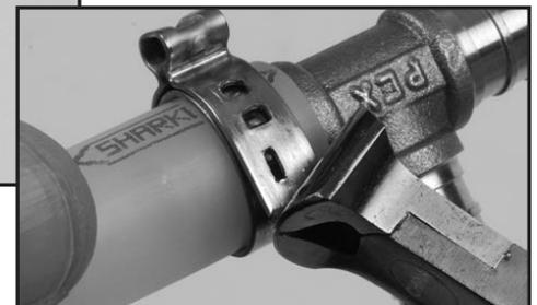
**Note:** The previously clamped section of SharkBite® tubing should be cut off prior to making a new connection.
