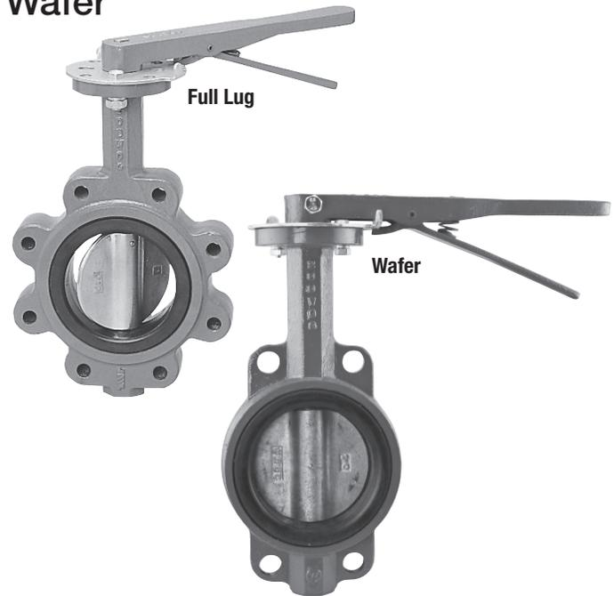
**Disc** – Disc edge is machined and polished 360° to assure leak-tight shutoff while minimizing operating torque. Positive, disc-to-shaft connection is provided by stainless steel precision taper pins that are vibration proof.
