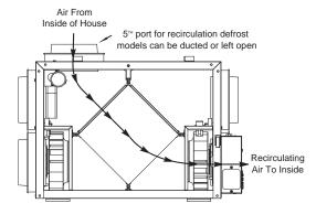
**INSTALLATION** Unit is typically hung by using installation kit supplied with unit. Mounting bolts provided on top four (4) corners of unit.
