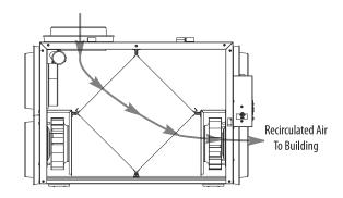
**INSTALLATION** Unit is typically hung by using installation kit supplied with unit. Mounting bolts provided on top four (4) corners of unit.
