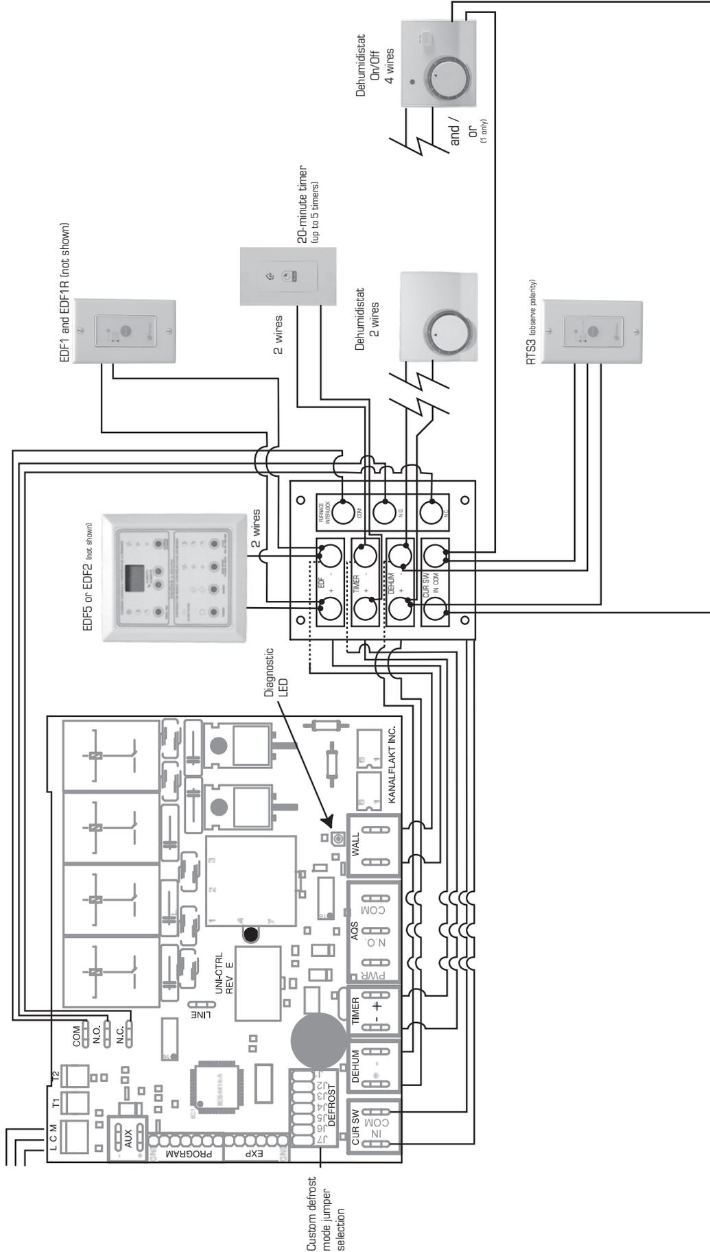
\* Wiring diagram of complete unit inside of access panel
