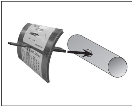
**1** Cut hole in duct and insert flow measuring station. Make sure that the flow measuring station's air direction arrow points in the direction of the airflow. Secure the flow measuring station with duct tape.
