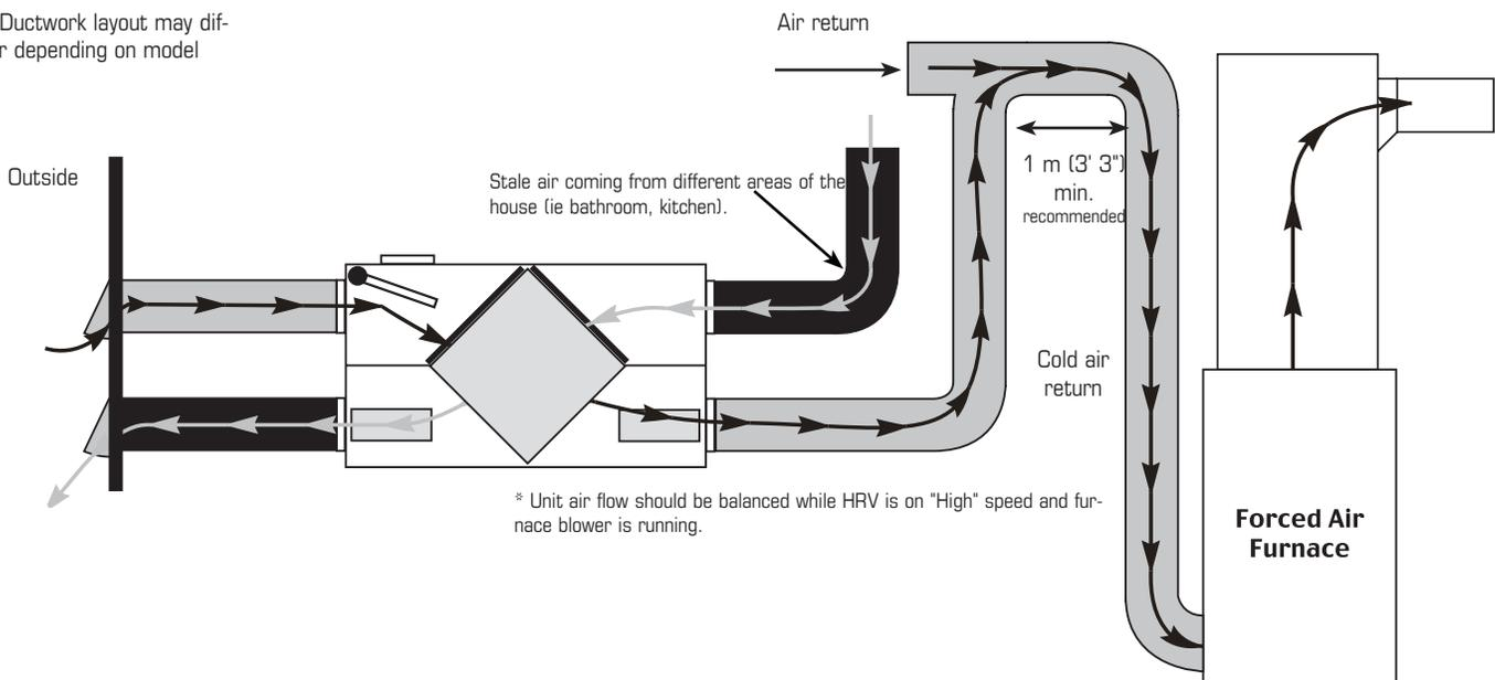
\* Unit air flow should be balanced while HRV is on "High" speed and furnace blower is running.
