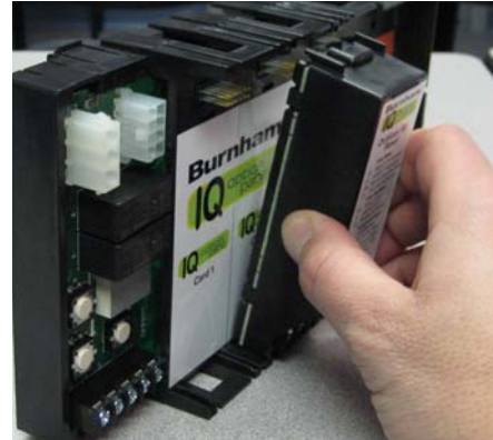
Insert IQ Option Card into selected slot
