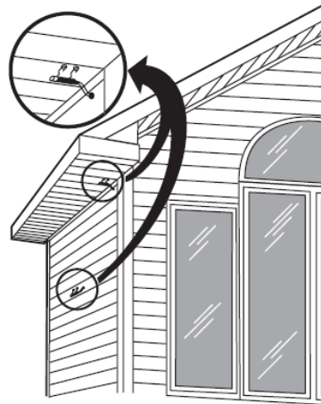
typical locations for outdoor sensor
