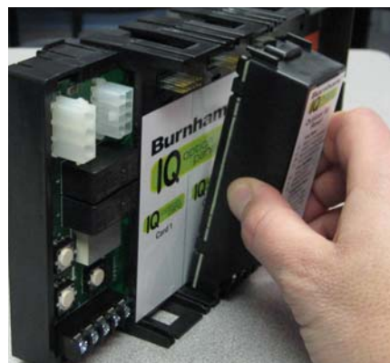
Insert IQ Option Card into selected slot
