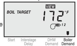
To view all control settings, the *Item* button may be pressed and held while in the View Menu. The control will then scroll through all the adjustable items.
