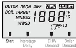
The control then automatically goes to operating mode, and displays the outdoor temperature.
