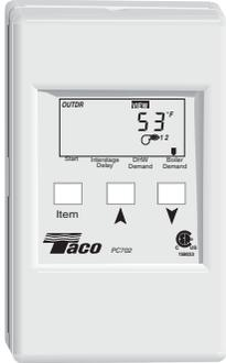
The PC702-1 is a microprocessor-based control designed to regulate the supply water temperature from a two stage boiler system based on the outdoor temperature or DHW requirements. A wiring harness is provided to be easily connected to the Taco Expandable (-EXP) Controls.
