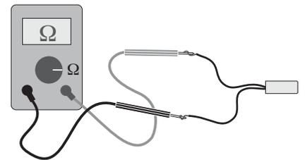
**Do not apply voltage to a sensor at any time as damage to the sensor may result.**
