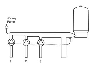
2. WELL-X-TROL® 440 through 460 Series are sometimes used on pressure regulation stations to provide system dampening during periodic high peak loading such as laundry wheels, etc.
