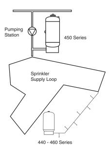
3. In a municipal well system or pressure boosting station, WELL-X-TROL®s are used to control sequential start of the main pumps. At the same time, it reduces surge and provides the jockey pump with guaranteed minimum run times during low peak demand periods.
