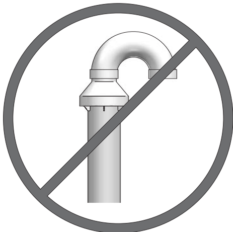
Figure 5-5 Do Not Install U-Bend to Rain Cap
