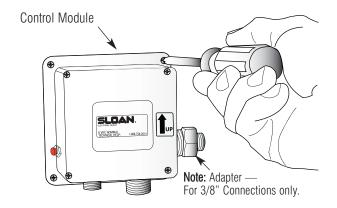
Install Control Module to wall using Fasteners supplied.
