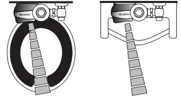
2. When the user enters the sensor's effective range, the Red LED light in the sensor window flashes for eight seconds. After eight seconds of sensing the user, the light will stop flashing and the unit waits for the user to step away before initiating a flush cycle.
