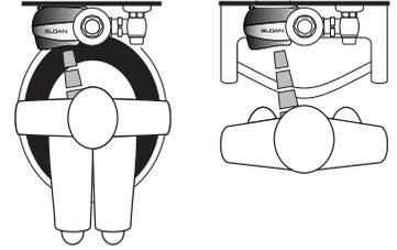
3. When the user steps away, the unit initiates a flush cycle. The unit then automatically resets and is ready for the next user.
