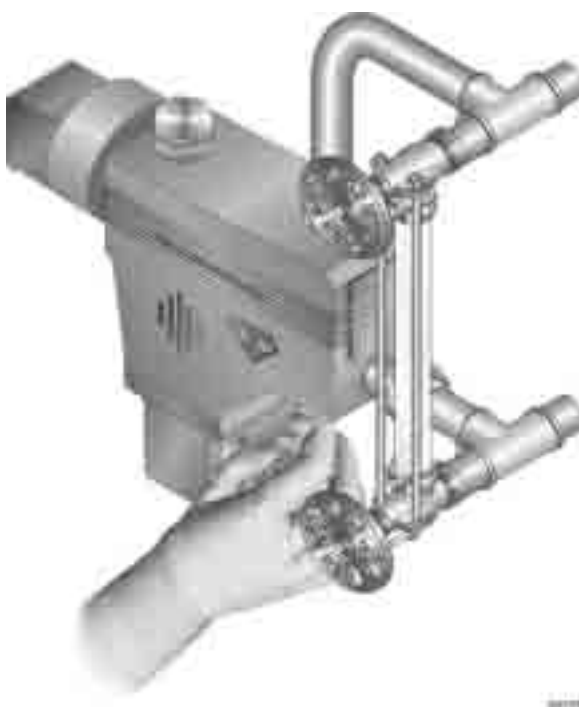
Figure 7 Float type low water cutoff
