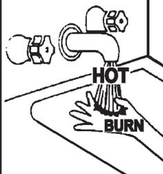
**▲ DANGER** Water temperature over 125°F (52°C) can cause severe burns instantly resulting in severe injury or death.
