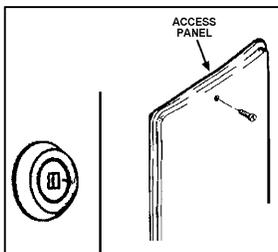
Caution: This access panel covers a 2" NPT plug that was required during the manufacturing of this water heater. This 2" NPT flange is **not** a cleanout fitting, removing the 2" NPT plug and using this fitting as a cleanout could void your warranty.
