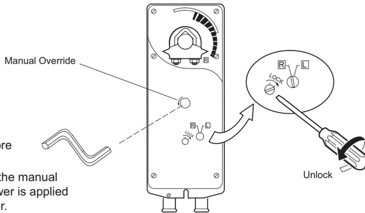
Fully engage hex wrench into manual override before winding.
