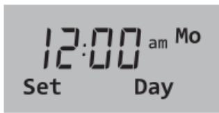
**NOTE:** The clock has lost its settings when the time display flashes. If the thermostat is following the schedule, it will use the temperature settings programmed for Period 1 of the weekdays until you readjust the clock.
