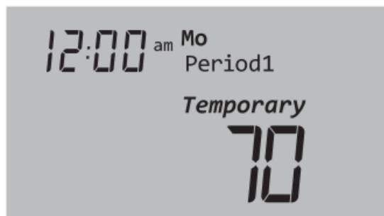
**NOTE:** Pressing the **Up** or **Down** button once will display the setpoint temperature. To change the setpoint temperature, press either button more than once.
