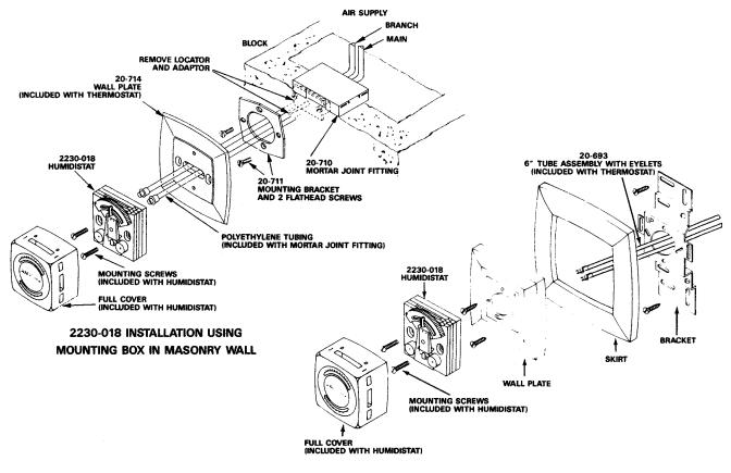
MOUNTED WITH 22-022 WALL PLATE & SKIRT (MOUNTING SCREWS INCLUDED WITH KIT)
