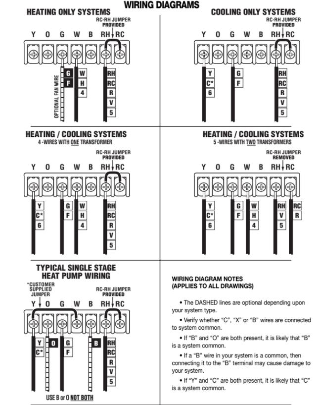
These diagrams below are provided for new installations or unreferenced wires.
