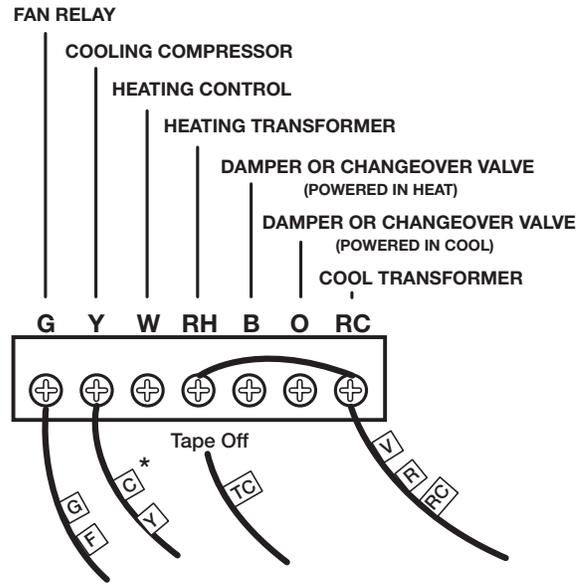
\* If both Y and C wire are present, tape off "C" wire.
