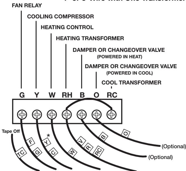
\* If both Y and C wire are present, tape off "C" wire.
