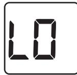
This condition could occur from the system being turned off during a cold weather period or upon installation when the thermostat has been stored for a long period of time in a cold vehicle or location prior to being installed. The thermostat should be allowed to warm up prior to installation to allow proper heating control once installed.
