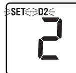
3. Press and hold the **▲** and **▼** buttons at the same time again and the LCD display will show "SET D2 x°", where "x" equals the °F / °C differential setting. This is the current second stage differential setting.
