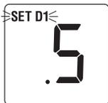
**NOTE—MODEL 1000, 1000NC:** Once you have finished setting the first stage differential, you can wait 5 seconds and the thermostat will return to the normal operating mode. Or you can press both the **▲** and **▼** buttons at the same time to return to normal operating mode.
