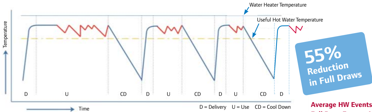
Hot-water Events — Insulated Pipes Average Daily Household Usage
