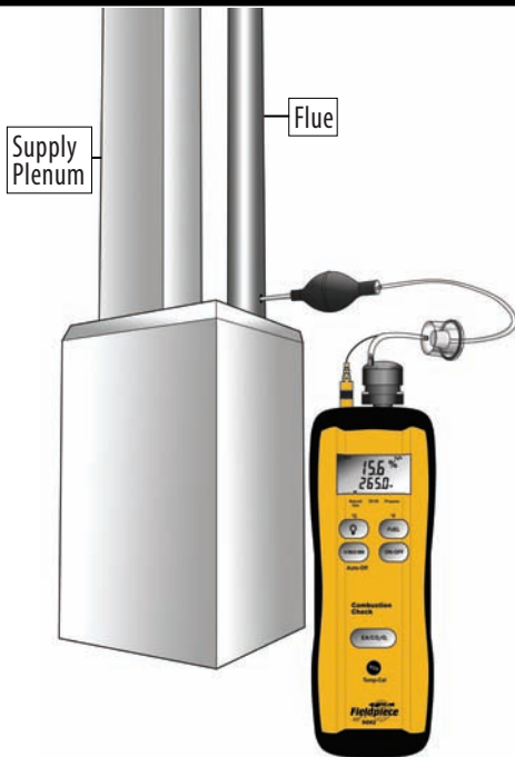
The Fieldpiece SOX2 measuring %O 2 and stack temperature inside a flue.
