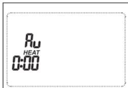
8. **Lockout (0-8°, NITE, COOL-HEAT)** – Select the number of degrees set temperature can be changed during keypad lockout or select to lockout during **NITE** period only. **COOL-HEAT** lockout allows adjustment of the set temperatures to the maximum heat set temperature selected in Step 9 and minimum cool set temperature selected in Step 10.
