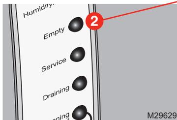
Wait for the Empty light to turn on. (It takes about 45 minutes for the tank to drain.) This indicates that the water has finished draining.
