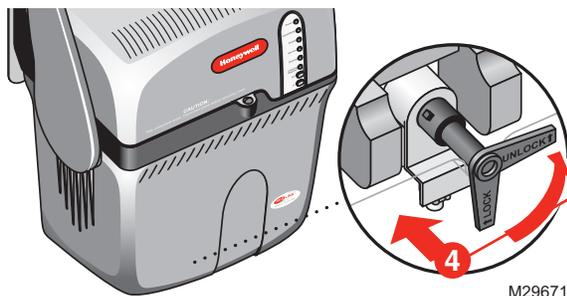
Turn the manual shutoff valve at the tank bottom to the “Unlock” position.
