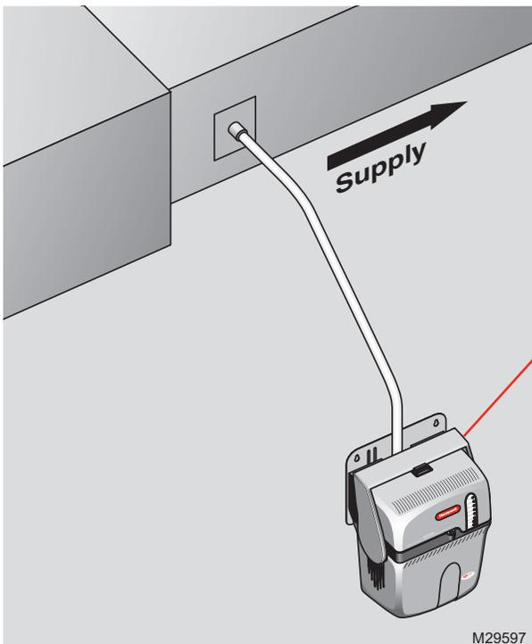
**Remote mounting.** TrueSTEAM is installed some distance away from your furnace supply duct. An insulated hose carries steam from TrueSTEAM to a suitable location on the supply duct.
