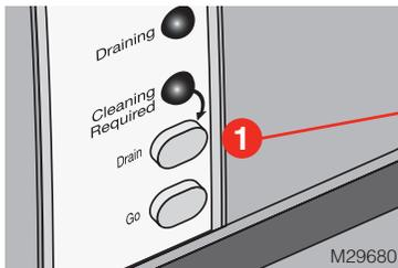
Press the Drain button to initiate a flush cycle and empty the water tank. You will know the tank is draining when the Draining light is blinking.
