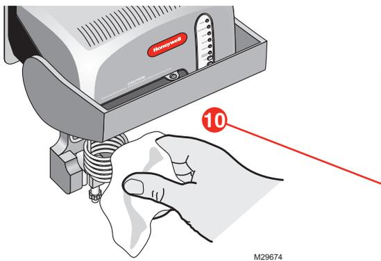
Unplug the TrueSTEAM, and carefully rub minerals off the heating element and reservoir walls.
