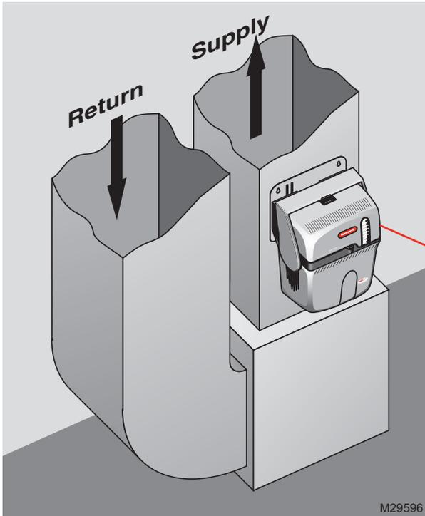
**Duct mounting.** TrueSTEAM is installed directly onto the supply (hot) air duct of your furnace. The steam nozzle sends steam directly from TrueSTEAM into the duct for distribution through your home.
