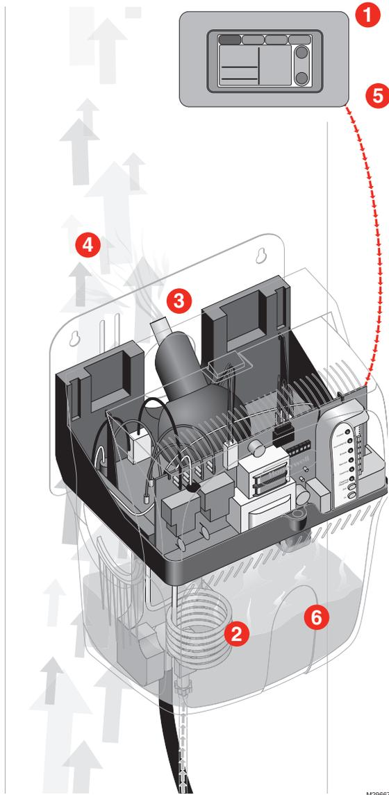
1. A call for humidity comes from the humidity control provided with TrueSTEAM. The humidity control is connected to TrueSTEAM, either with wires or by wireless connection.
