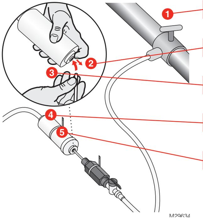
1 Turn the water supply off at the saddle valve or T-fitting and manual shutoff valve.
