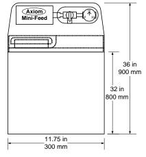
Depth - 11.75 in 300 mm Clearances – Right Side and Top - 12 in 305 mm Discharge 1/4" FPT
