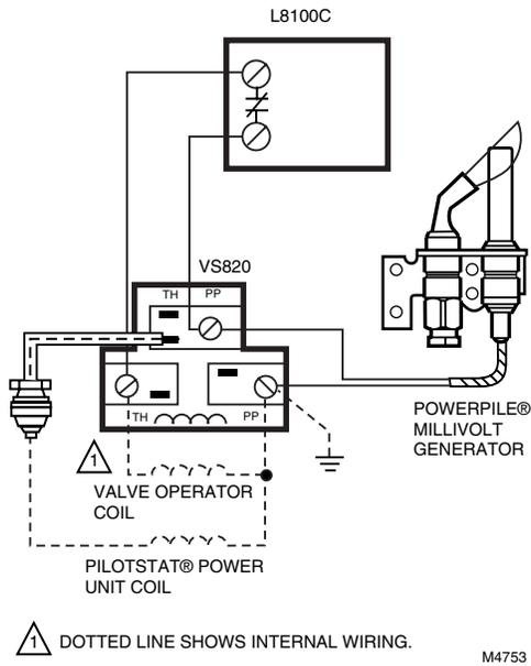
Fig. 11. L8100C hookup with three-terminal VS820 to cut out main valve.
