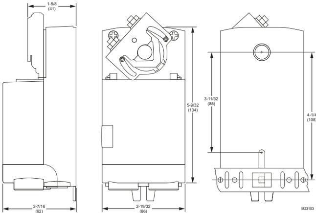
Fig. 1. Dimensional drawing of actuator in in. (mm).
