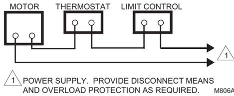
**Fig. 6. Typical connections for Series 41 Motors.**
