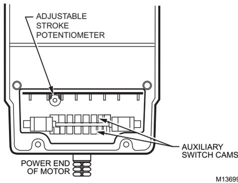
**Fig. 11. Stroke adjustments.**
