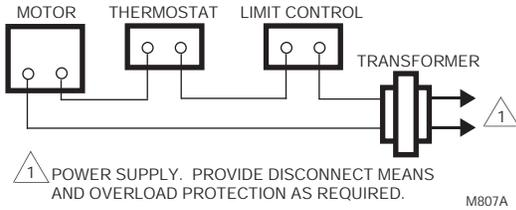
**Fig. 7. Typical connections for Series 81 Motors.**
