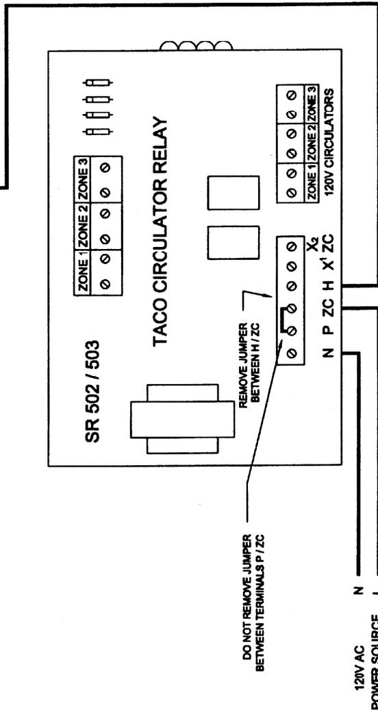
**Note:** This drawing is conceptual in nature and does not purport to address all design, installation or safety considerations. Additional safety and/or auxiliary equipment may be needed. This diagram is for reference use by officials, designers and licensed installers. It is expected that installers have an adequate knowledge of accepted industry practices for the equipment, procedures and applications involved.
