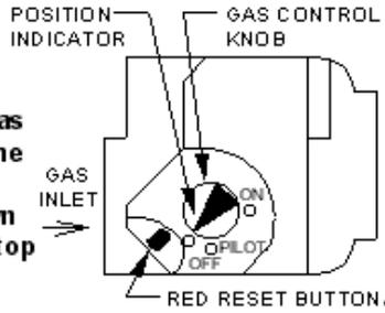
8. Rotate gas control knob clockwise from "ON" position to "OFF" position.
