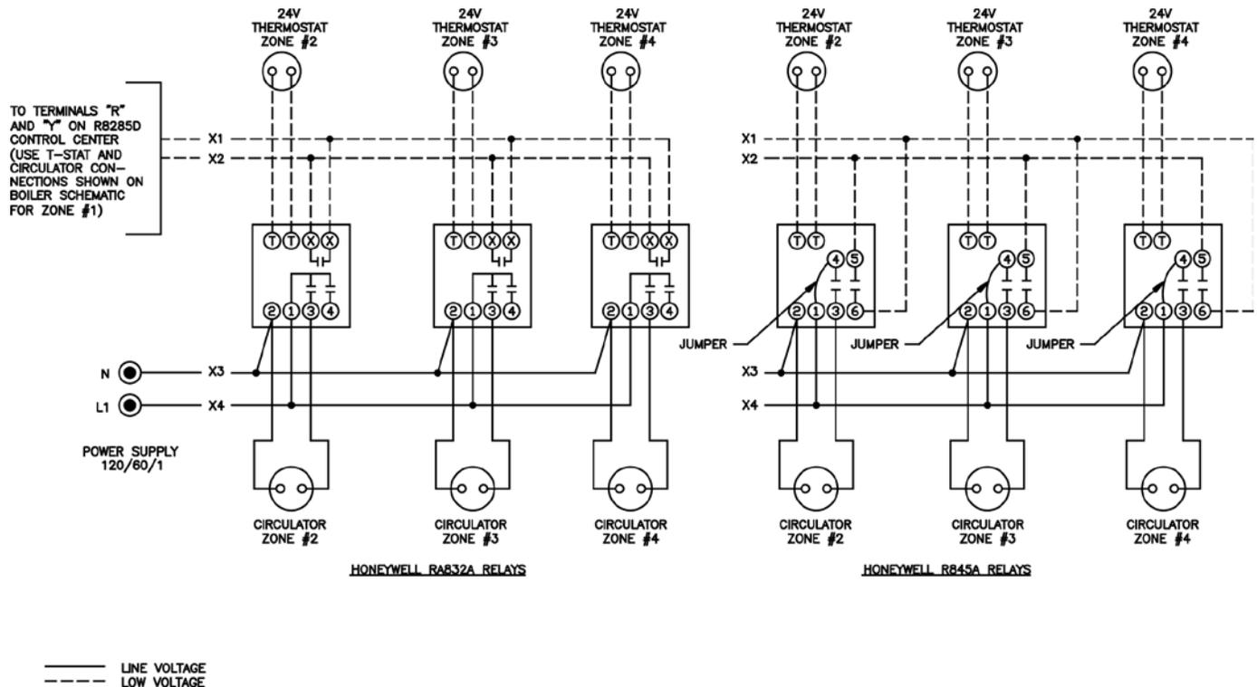
**Figure 16: Wiring Schematic, Zone Circulators**
