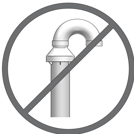
Figure 5-5 Do Not Install U-Bent to Rain Cap
