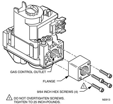
form on the control after completing the installation includes leak testing the adapters and screws. If you use a wrench on the gas control after flanges are installed, use the wrench only on the flange, not on the control.
