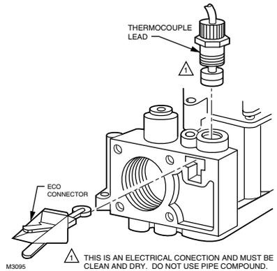
**Fig. 8—Wiring connections.**
