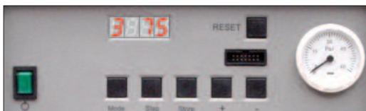
A 4-digit user's Interface Module is provided to display system operating status and fully adjustable parameter values as well as diagnostic codes for easy troubleshooting and optimum system performance.
